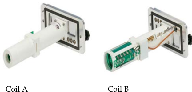
Figure 12: Radio Frequency (RF) coils (A) is 35mm and (B) is 60mm coils
